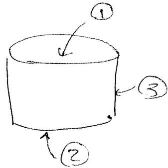
$$\begin{aligned} \text{surface 1: } & \sigma_p = P_0 \\ \text{surface 2: } & \sigma_p = -P_0 \\ \text{surface 3: } & \sigma_p = 0 \end{aligned}$$
